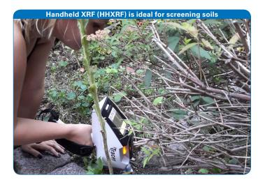
Portable XRF Elemental Analyzers: Simultaneously measure elements from sodium (Na) to uranium (U) at concentrations as low as parts-per-million to high percentage levels (depending on the element). Objects of any form – liquid, solid, cores, powder, sludge, slurries, filters, wipes, chips – can be analyzed wherever they are located.
